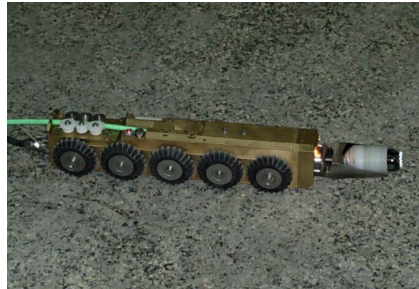
Fig. 10: Prototype of a satellite camera for use in pipes up to DN 135
