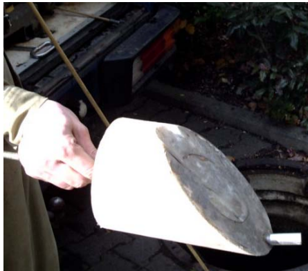
Fig. 16: Insert wedge used as an aid for condition assessment by optical inspection
