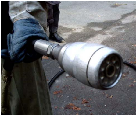
Fig. 11: High flushing pressure camera
