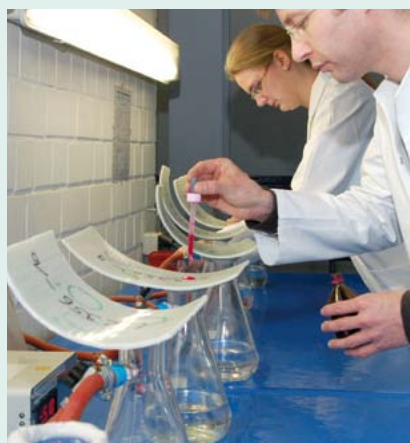
Tightness testing of tube liners
