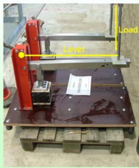
IKT: Interaction between roots and elastomeric material
